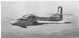
LARGE SPEED BRAKE is extended hydraulically under Cessna T-37A's nose. Cockpit canopy can be jettisoned by explosive charges.
